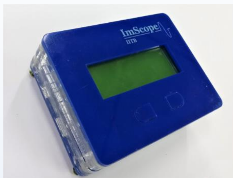
Standalone Electrochemical Impedance Spectroscopy based system for health and environment.
